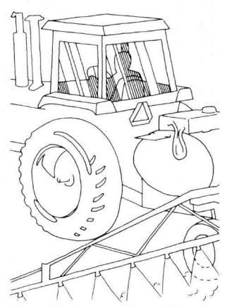
**Figure 11** Tractor cabs provide excellent operator protection from chemical application exposure.
