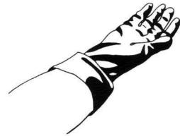
**Figure 6** Gloves must be chemical resistant, unlined and waterproof.
