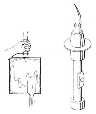
Figure 15 A jet rinse for rinsing chemical containers.
