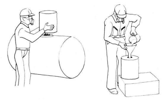
Figure 14 Triple rinse containers to remove residue.
