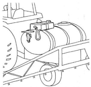
Figure 10 Example of a sprayer with glove holder and auxillary water tank for cleanup.
