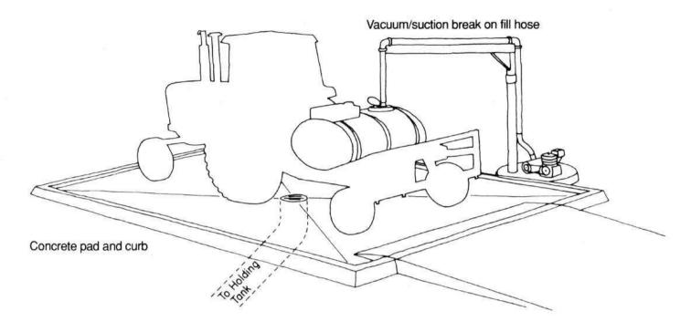
Figure 12 Containment loading area.
