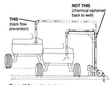
**Figure 13** Prevent backsiphoning by providing a vacuum break.
