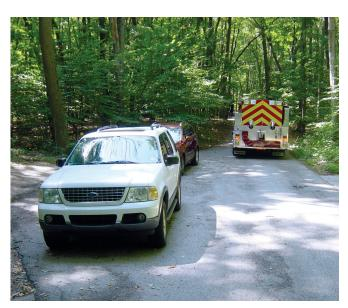
**Figure 3.** Passing areas on narrow lakeshore private roadways such as this one near Grand Haven, Mich., allow emergency vehicles to pass. (*Courtesy of Grand Haven Township Fire and Rescue*)
