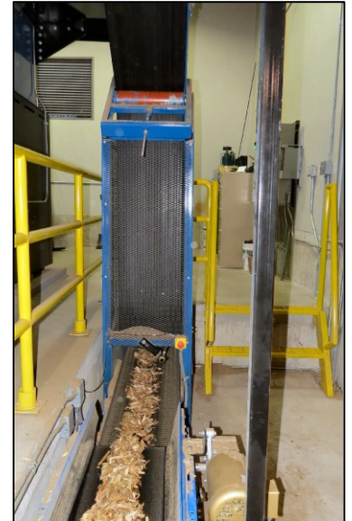
Walking auger pulls chips to a conveyor. Chips are lifted by a vertical conveyor, prior to feeding into the combustion chamber.
