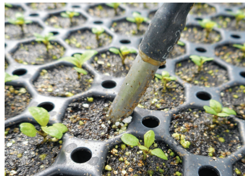
Figure 2. Substrate temperature is measured by a thermistor connected to an environmental control computer.
