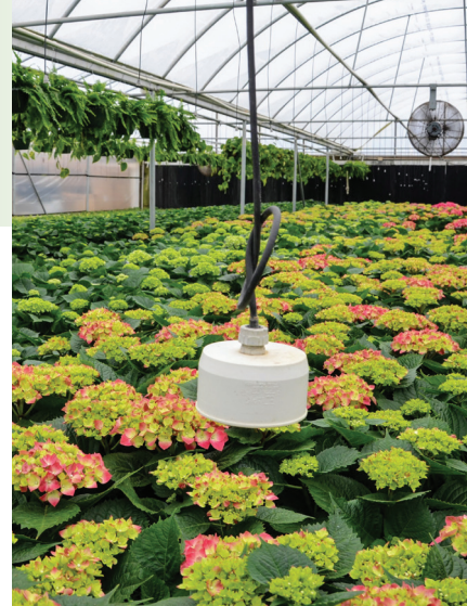
Figure 1. Greenhouse air temperature is measured at plant canopy height by fan-driven aspirated thermistors connected to an environmental control computer. Photos by W. Garrett Owen.
