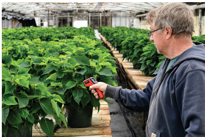
Figure 4. Mark Watkins of Bogie Lake Greenhouses in White Lake, MI, uses a calibrated hand-held infrared (IR) thermometer equipped with a laser to measure poinsettia leaf surface temperature.
