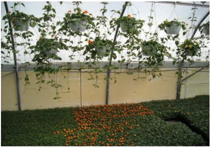
Insulation of the greenhouse perimeter saves heat.
