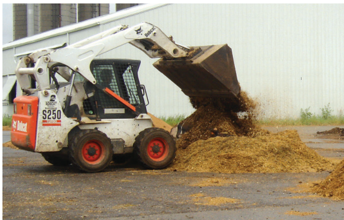
Photo 4. Covering the carcass and shaping the new pile.
