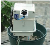
Figure 4. An external quantum sensor attached to a data-logging computer program.
