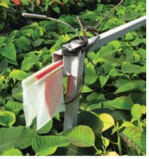
Figure 2. A temperature sensor properly placed above a canopy of poinsettias.
