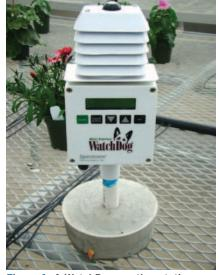
Figure 1. A WatchDog weather station manufactured by Spectrum Technologies containing built-in air temperature and quantum sensors.
