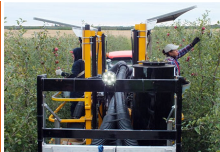
Workers demonstrating an innovative tractor-pulled hydraulic platform apple harvester in a high density apple orchard.
