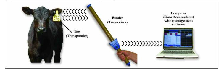
Figure 1. The four basic components of an RFID individual management system.
