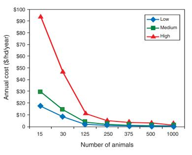
Figure 2. Annual costs for example RFID-based individual animal management systems (defined in Table 5) as affected by number of animals managed. Reader and data accumulator values depreciated over 4 years; software depreciated over 5 years. Graph was generated using a spreadsheet developed by K.C. Dhuyvetter and D. Blasi and is available at <u>http://www.beef</u> stockerusa.org/rfid/index.htm.
