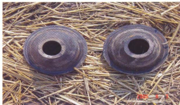
The rubber cone on the right has been slightly trimmed to increase flow.
