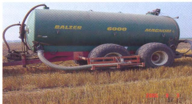
The basket attached to the side of the spreader provides easy access to the hose used to transfer manure from the farm's 6,000 gallon nurse tanks.
