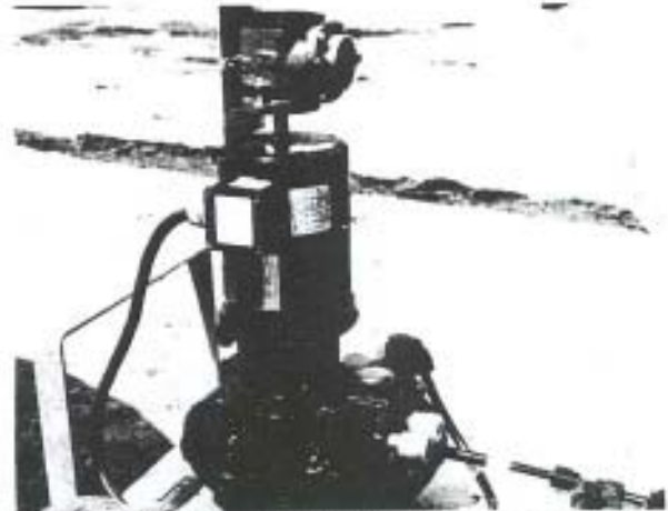
Low maintenance and ease of adjustment are among advantages of diaphragm pump.
